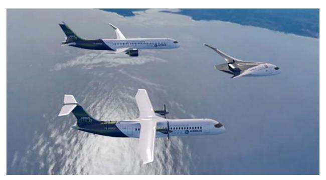
The three ZEROe concepts program include a 120-200 passenger turbofan with a range of 2,000+ nautical miles, capable of operating transcontinentally and powered by a modified gas-turbine engine running on hydrogen. The liquid hydrogen will be stored and distributed via tanks located behind the rear pressure bulkhead.
